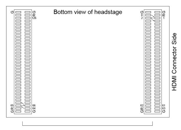
Hirose DF40 70-pin connectors, 25.0 mm apart (center to center). Mating connector: *Hirose DF40C-70DP-0.4V(51)*
