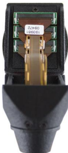
Figure 2 | Neuropixels Probes connected to cone assembly via tiered zero insertion force (ZIF) connector interface.
