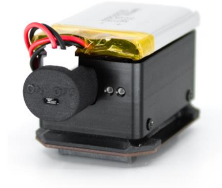
Figure 5 | HH128 logger and base with mounted battery and micro HDMI battery connector.
