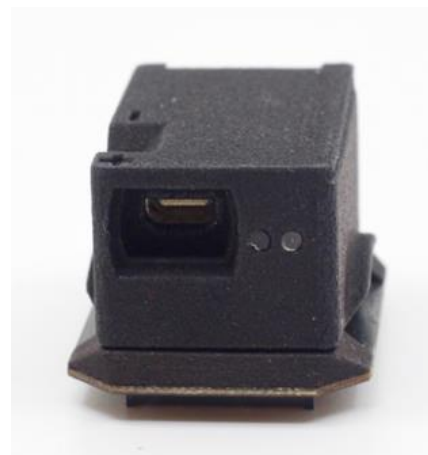
Figure 3 | Side view showing LED indicators to the right of the HDMI port and Mill-max polarity designations indicated by plus (+) and minus (-), where power (+) is the pin closest to the HDMI port.
