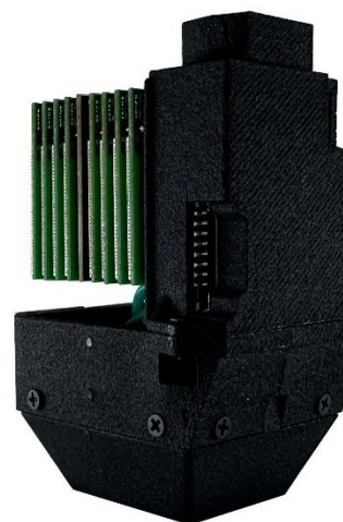
Figure 1 | MSH with open module bay. 8 128-channel Probe Boards (green) and 1 reference board (black).
