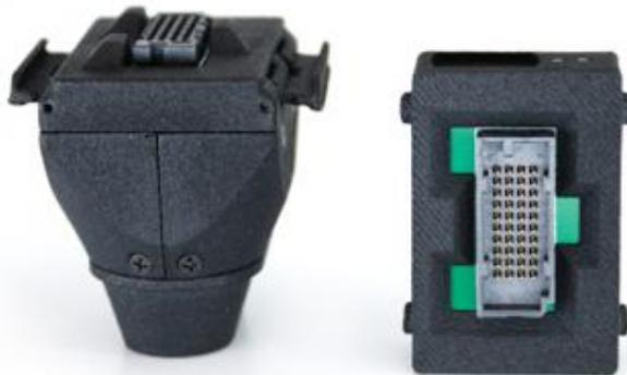
**Figure 1** | Neuropixels Headstage cone assembly (left) and removable data-logging headstage (right). Data-logging headstage shown from bottom, with connection interlock and Samtec connector.
