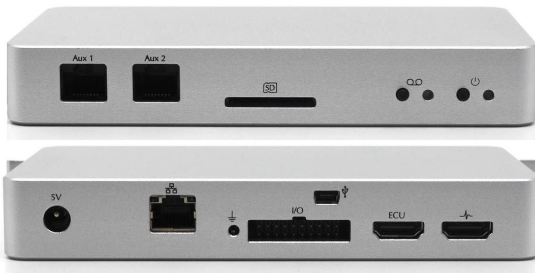
**Figure 1** | The MCU front (top) and rear (bottom) panels.
